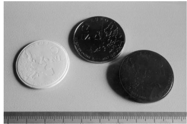
Fig. 8. Comparison of the stamping die (in the middle) green body (right) and sintered ceramic (left).
